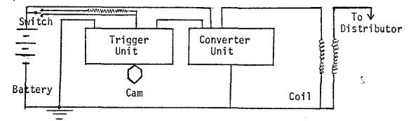
The sensor is a magnetic pulse generator whose pulses are generated by movement of the distributor cam in the magnetic field. This signal is fed into the capacitive discharge circuit discharging the storage capacitor into the primary windings of the ignition coil. The capacitive discharge circuit consists of a d-c converter, storage capacitor and an electronic switching circuit. The system is capable of an output of 32 KV and 60 millijoules according to manufacturer.
