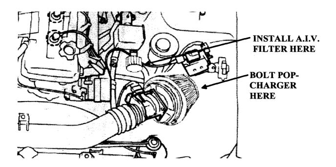
NOTE : SOME MODELS MAY BE SUPPLIED WITH A AMBIENT AIR TEMPERATURE SENSOR ATTACHED TO THE ORIGINAL AIR BOX. RELOCATE THIS SENSOR NEAR THE AIR FILTER INLET WITH THE ZIP TIE PROVIDED.
