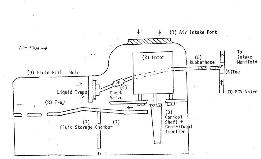
Figure 1 - Schematic of "Manfredi Fuel Booster"
