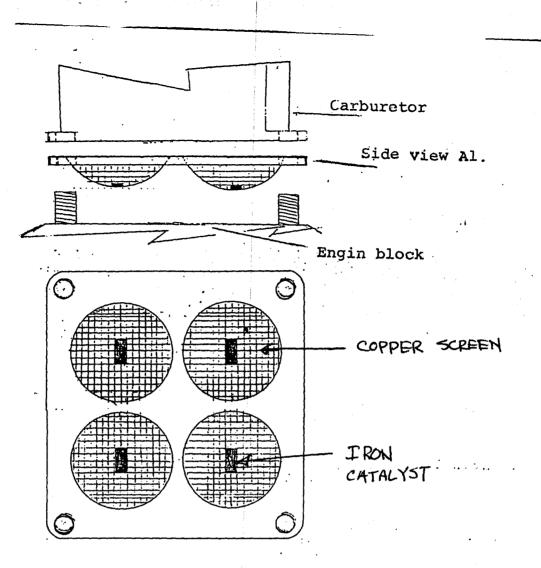
Al. fits between carburetor and engin letting a mixed air and gas pass through.
