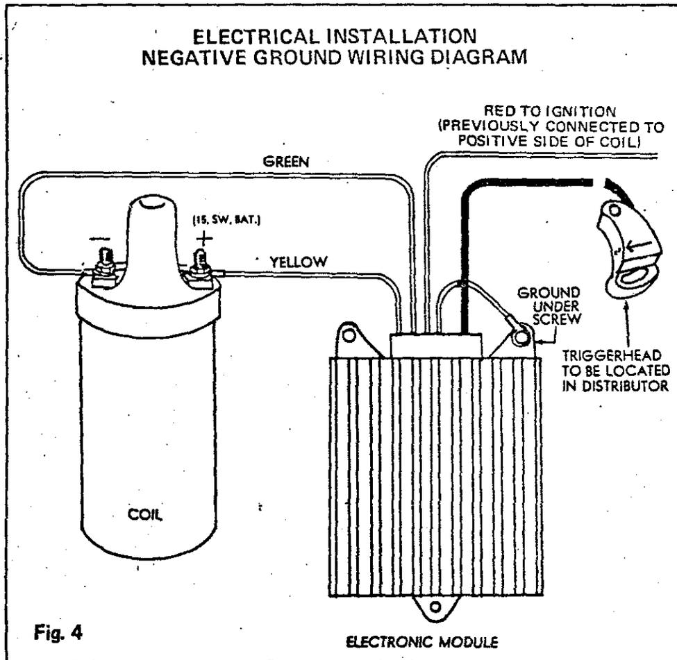
as above. Resistors and radio interference capacitors are not required and should be disconnected from the coil.
