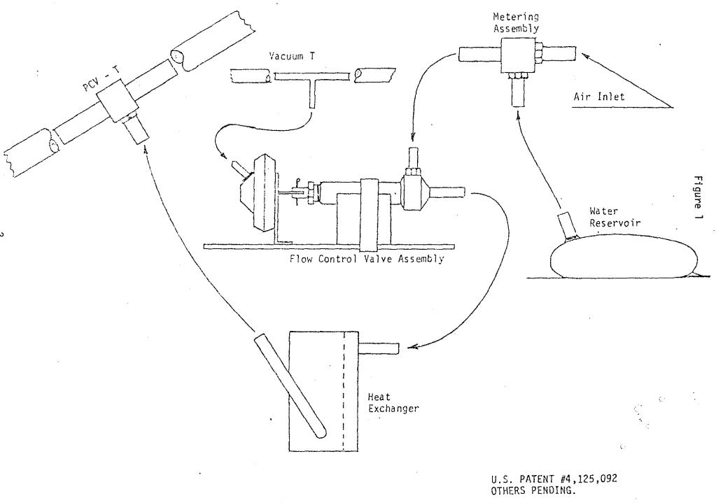
Once the location of the water reservoir, and the proper air and water orifices are determined for a given vehicle, the flow of water/air mixture is controlled by a spring-loaded tapered needle in the flow control valve operated by ported vacuum.
